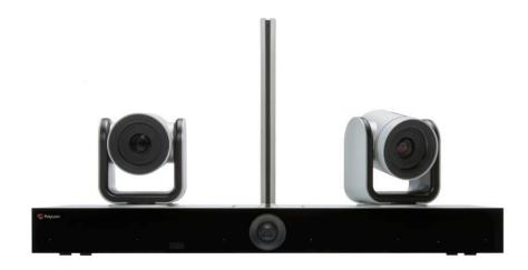
You can use the camera as a USB camera in the Bring Your Own Device (BYOD) mode, connect to a RealPresence Group Series system in the Group Series mode, or let the camera automatically detect a connection.
