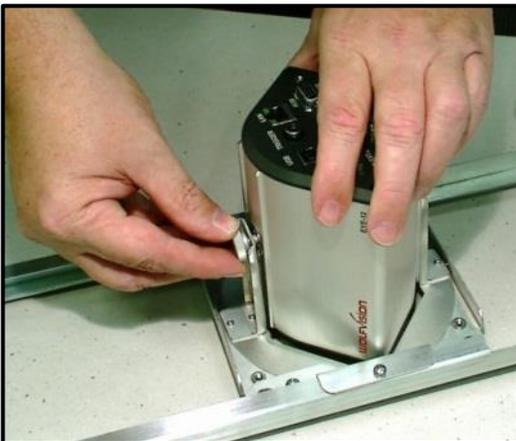
9) Install camera into the assembly – tighten  $\frac{1}{4}$  - 20 knurled screws (supplied with camera).
