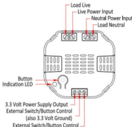
**Note:** The electricity to the circuit must be shut off during installation for safety and to ensure that wires are not shortcircuited during installation, which will cause damage to the Micro Module.
